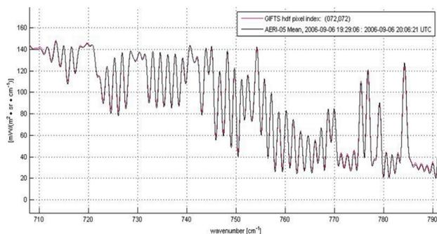
**Fig. 11.** Comparison of AERI and GIFTS  $\text{CO}_2$  region spectra observed at Logan UT on 6 September 2006.
