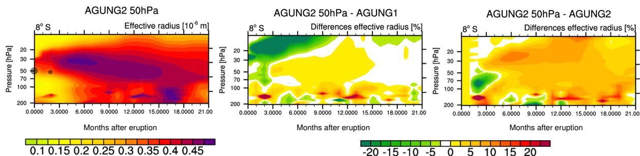
Figure 2: Hovmöller diagram of monthly mean effective radius  $\mu\text{m}$  of sulfate at the grid point corresponding to  $8^\circ\text{S}$ . Left: Simulation with two eruptions at the same height. Middle: Difference to AGUNG1. Right: Difference to AGUNG2. X-axis shows time after eruption.
