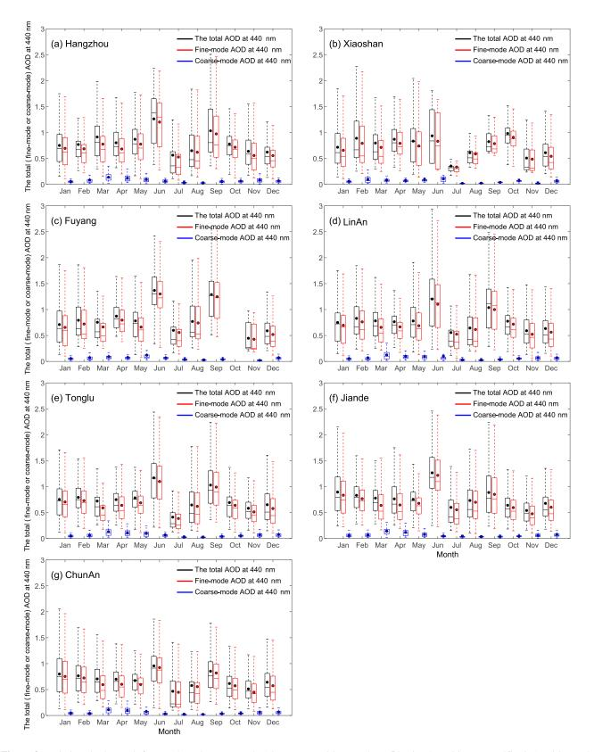
**Figure 3.** Variations in the total, fine-mode and coarse-mode AOD<sub>440 nm</sub> at (a) Hangzhou, (b) Xiaoshan, (c) Fuyang, (d) LinAn, (e) Tonglu, (f) Jiande and (g) ChunAn. The boxes represent the 25th to 75th percentiles of the distributions while the dots and solid lines within each box represent the means and medians, respectively.
