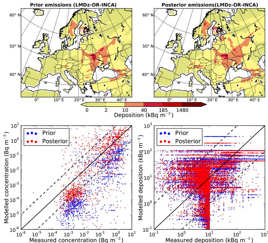
**Figure 10.** Deposition of  $^{137}\text{Cs}$  using the Eulerian LMDz-OR-INCA chemistry transport model prior emissions from the ensemble of six a priori releases and the optimized emissions resulting from our inversion. Comparison of modeled surface concentrations and depositions of  $^{137}\text{Cs}$  with observations from a recently published data set (Evangeliou et al., 2016).
