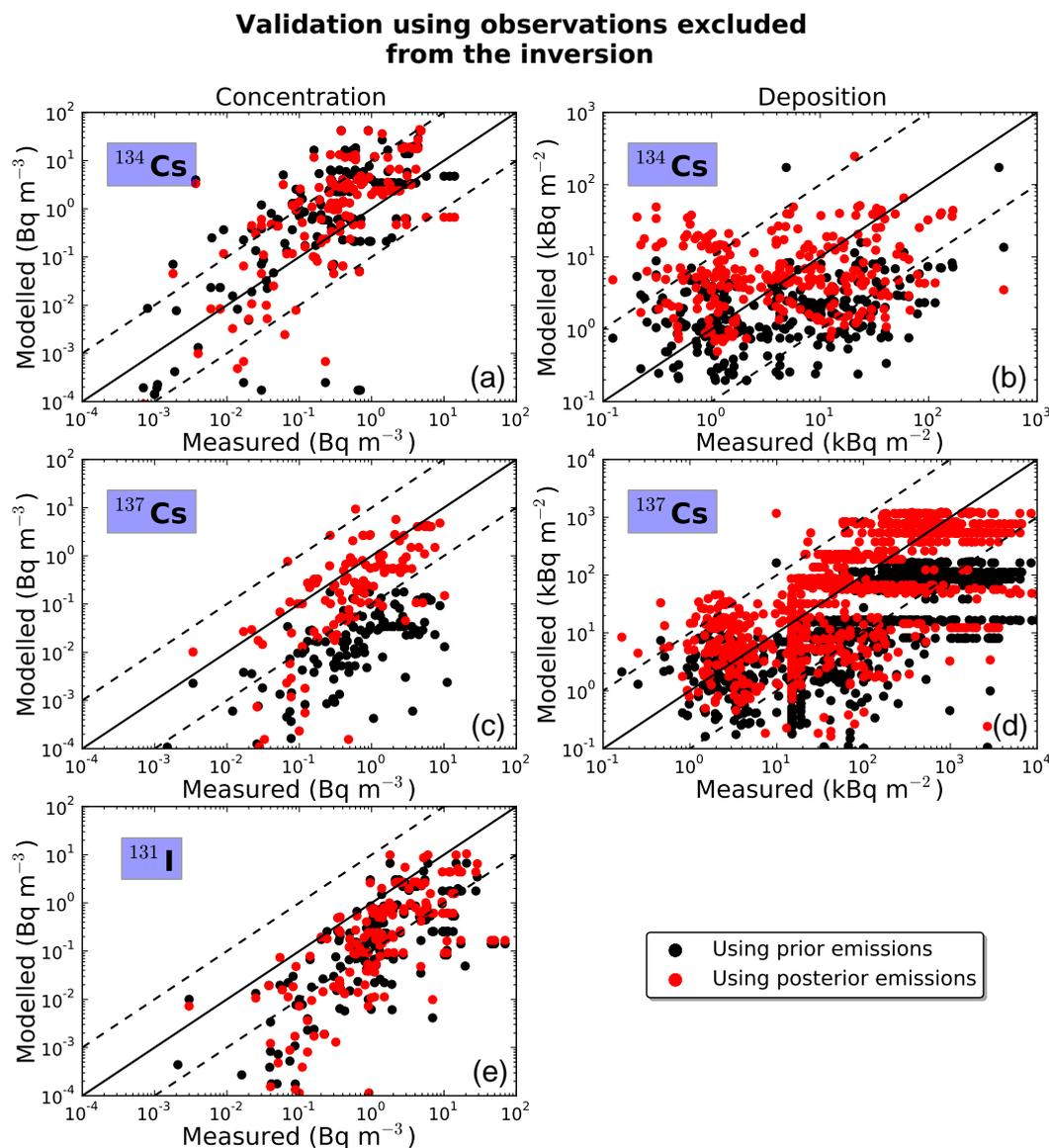
**Figure 7.** Left column: comparison of modeled concentrations with observations excluded from the inversions for  $^{134}\text{Cs}$  ( $N_{134} = 318$ ),  $^{137}\text{Cs}$  ( $N_{137} = 232$ ) and  $^{131}\text{I}$  ( $N_{131} = 318$ ). Right column: comparison of modeled deposition densities with observations excluded from the inversions for  $^{134}\text{Cs}$  ( $N_{134} = 273$ ) and  $^{137}\text{Cs}$  ( $N_{137} = 1115$ ).
