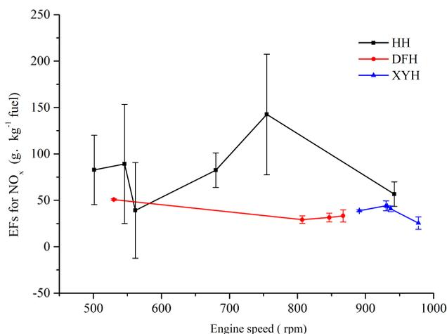
Figure 4. Emission factors for NO<sub>x</sub> at different engine speeds.
