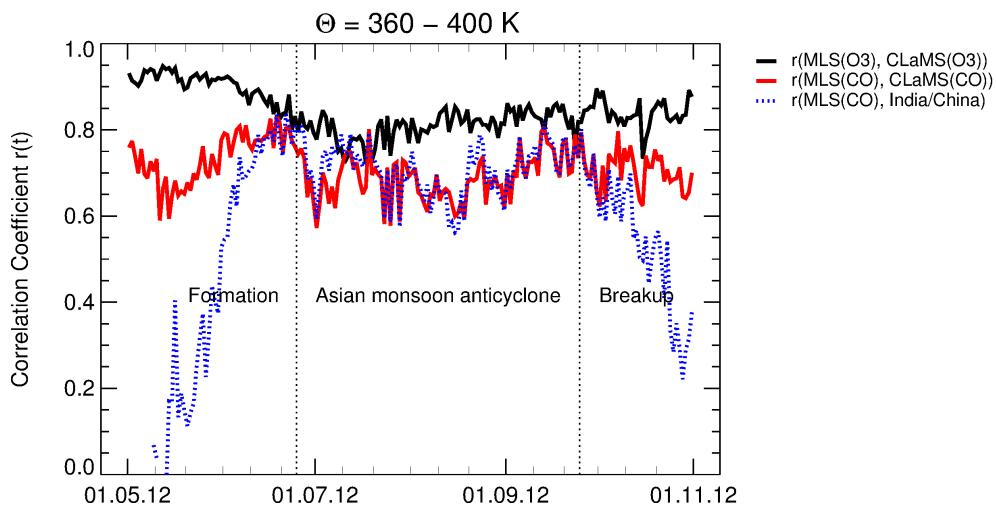
**Figure 4.** Correlation coefficients depending on time for tracer correlations patterns between MLS O<sub>3</sub> and CLaMS O<sub>3</sub> (black), between MLS CO and CLaMS CO (red), and between MLS CO and the CLaMS emission tracer for India/China (blue) for levels of potential temperature between 360 and 400 K (see text for more details) in a region between 15 and 50° N and 0 and 140° E (shown as black rectangles in Fig. 2 and 3).
