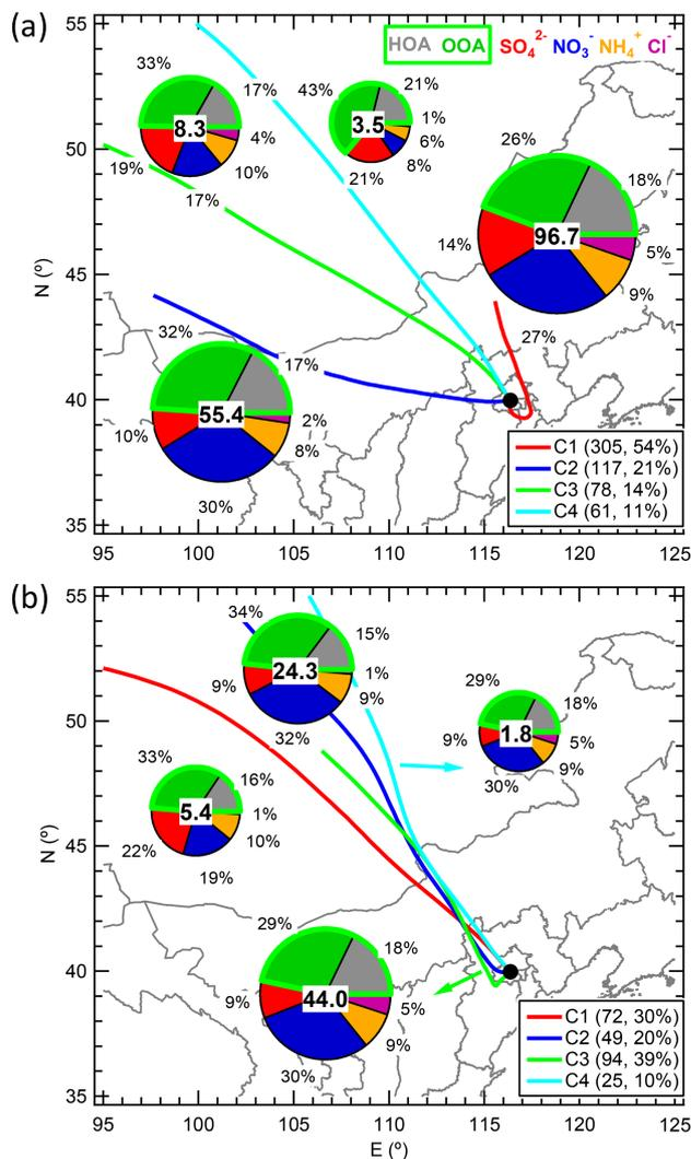
**Figure 10.** The average NR-PM<sub>1</sub> composition for each cluster (a) before and (b) during APEC. The numbers on the pie charts refer to the average total NR-PM<sub>1</sub> mass for each cluster. In addition, the number of trajectories and corresponding percentages of the total trajectories are also shown in the legends.
