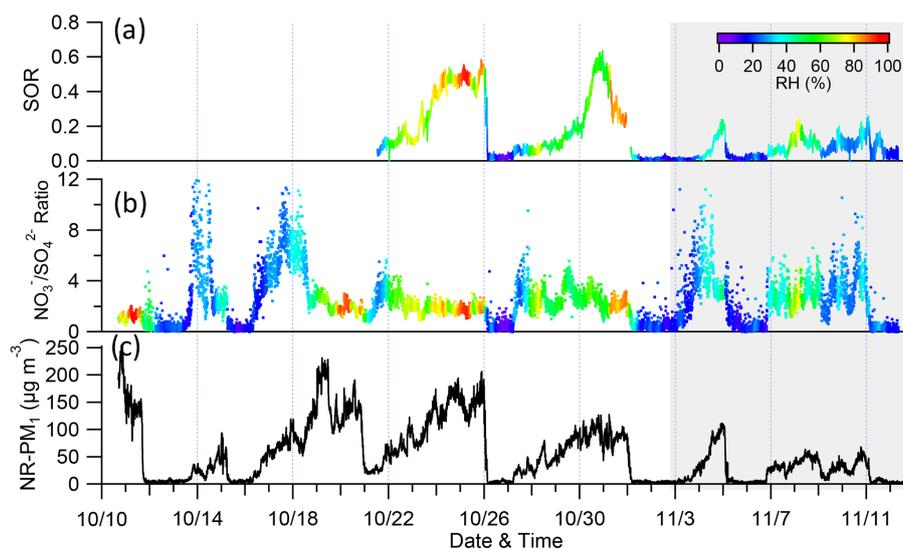
**Figure 3.** Time series of (a) sulfur oxidation ratio (SOR), (b) ratio of  $\text{NO}_3^-/\text{SO}_4^{2-}$ , and (c) NR-PM<sub>1</sub>. The SOR and  $\text{NO}_3^-/\text{SO}_4^{2-}$  were color-coded by RH.
