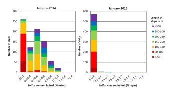
**Figure 3.** Sulfur fuel content in autumn 2014, and in January 2015, after the change of fuel regulations. The lengths of the ships that have been analysed are colour-coded. While in 2014 only small ships had fuel sulfur contents below 0.2%, nearly all ships fell into this category in January 2015.
