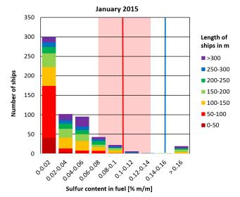
**Figure 4.** Detailed view of the January 2015 data set. The lengths of the ships are colour-coded; the red line indicates the 0.1 % limit, with the shaded area representing the upper limit uncertainty of 30%. The blue line indicates the suggested limit of 0.15% for flagging ships as exceeding the sulfur fuel content limit allowed.
