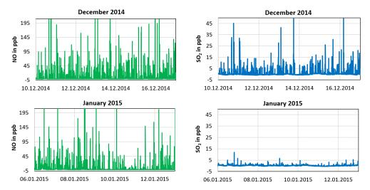
**Figure 2.** Comparison of absolute NO and SO<sub>2</sub> volume mixing ratio values measured over 2 weeks, 1 week in December 2014 and 1 week in January 2015 with comparable wind conditions. Each peak belongs to one emission plume of an individual ship. The reduction in SO<sub>2</sub> in 2015 is obvious, while for NO, no reduction can be observed.
