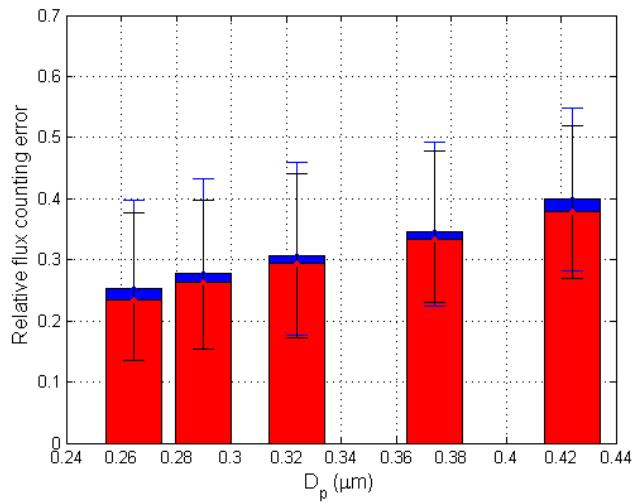
**Fig. 2.** Median relative counting error (bars) in particle flux for the five first OPC channels during the wet (blue) and dry (red) season. Error bars represent 25 and 75 percentiles of the counting error in the wet (blue) and dry (black) season
