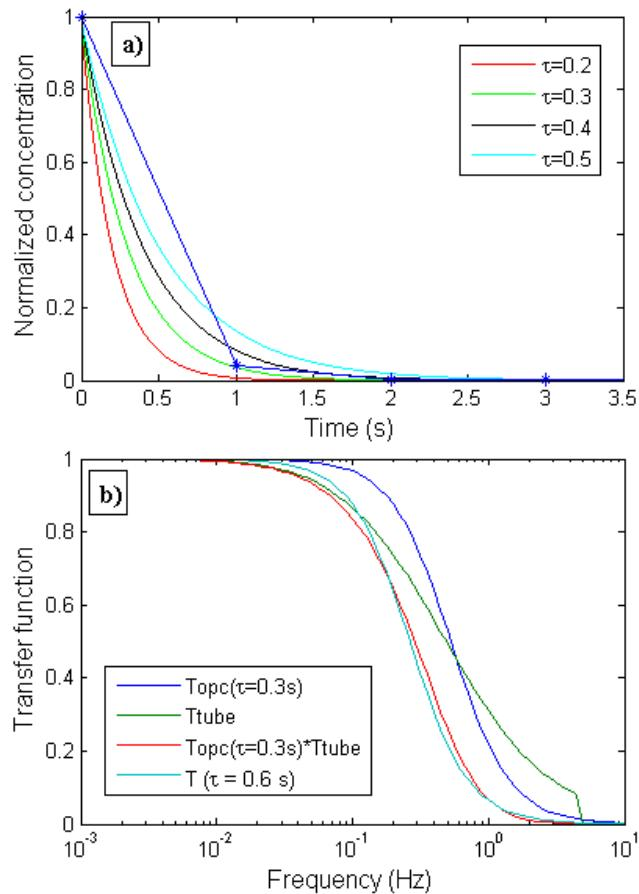
**Fig. 1.** (a) Time response of the Grimm 1.109 for a step decrease in particle concentration (blue) and time response curves for different values on  $\tau$  (Doebelin, 1990). —bf(b) Cospectral transfer functions for the OPC (Horst et al., 1997) (blue), tube (Lenschow and Raupach, 1991) (green) and in total (red) compared with a cospectral transfer function (Horst et al. 1997) for  $\tau = 0.6$  (cyan).
