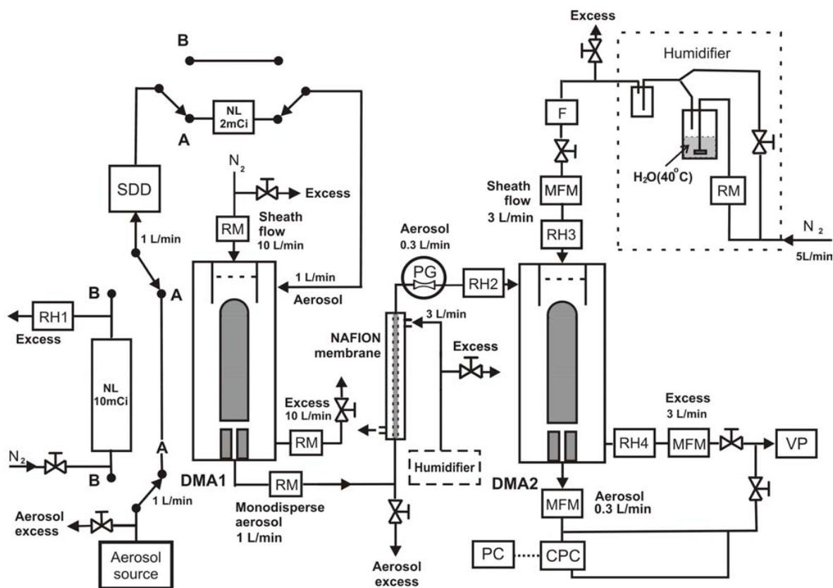
**Fig. 1.** Experimental setup of the hygroscopicity tandem differential mobility analyzer (H-TDMA) system: RH - relative humidity sensor, NL - aerosol neutralizer, SDD - silica gel diffusion dryer, RM - rotameter, DMA - differential mobility analyzer, PG - impactor and pressure gauge, MFM - mass flow meter, F - filter, CPC - condensation particle counter, PC - personal computer, VP - vacuum pump.
