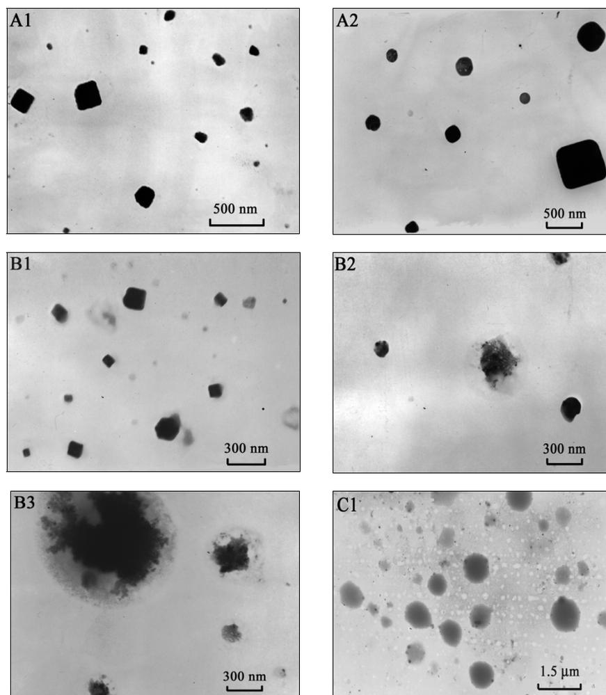
**Fig. 6.** TEM micrographs of deposited aerosol particles composed of sodium chloride (NaCl, high contrast) and bovine serum albumin (BSA, low contrast): pure NaCl particles before conditioning (A1) and after conditioning at  $RH=70\%$  (A2); mixed BSA-NaCl particles with BSA dry solute mass fractions of 25% (B1) and 50% (B2, B3); pure BSA particles (C1).
