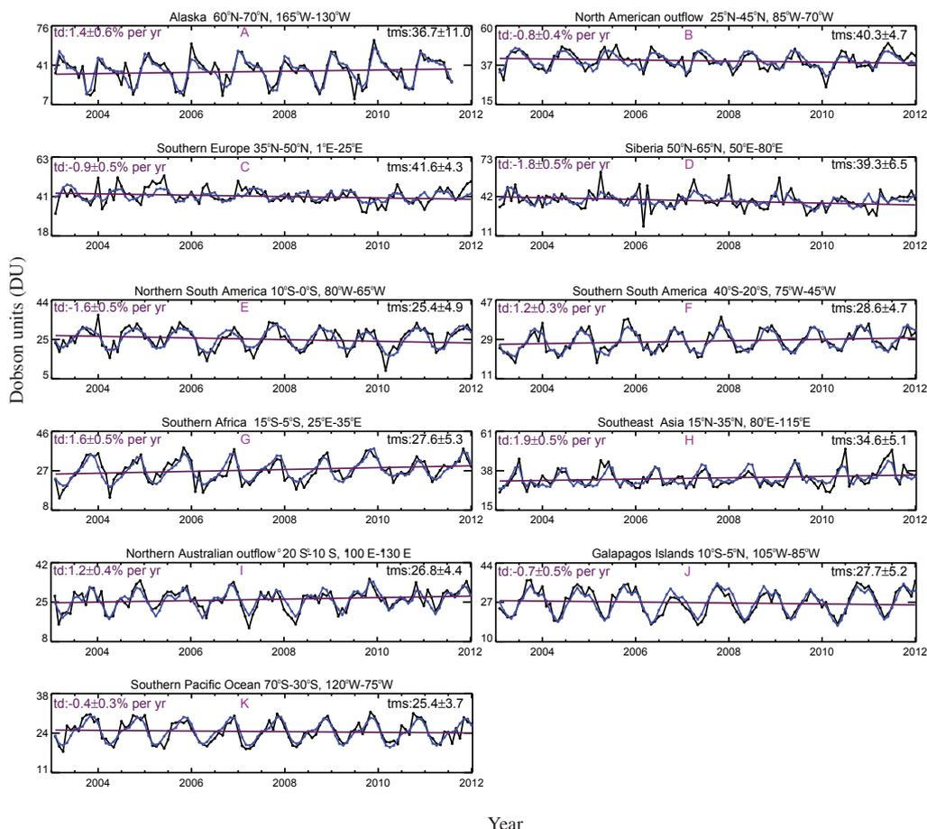
**Figure 12.** Time series (in Dobson units (DU)) (black) from SCIAMACHY (for the different regions A–K shown in Figs. 10 and 11) with overlaid fitting curves (blue) and linear change plus offset (violet) for the period 2003–2011.
