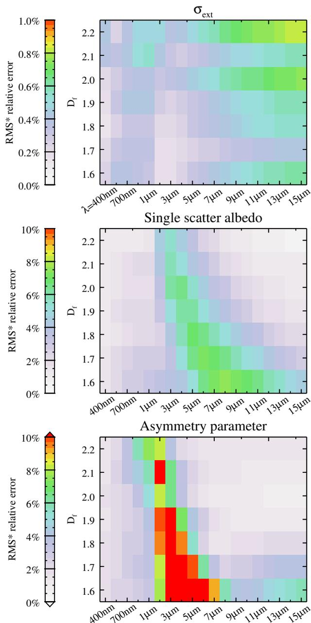
**Figure 10.** The relative RMSEs between the calculated and parameterised values of  $\sigma_{\text{ext}}$ , SSA, and  $g$ . Calculations of rms exclude the lowest two values of  $n_s$  as discussed in the text.
