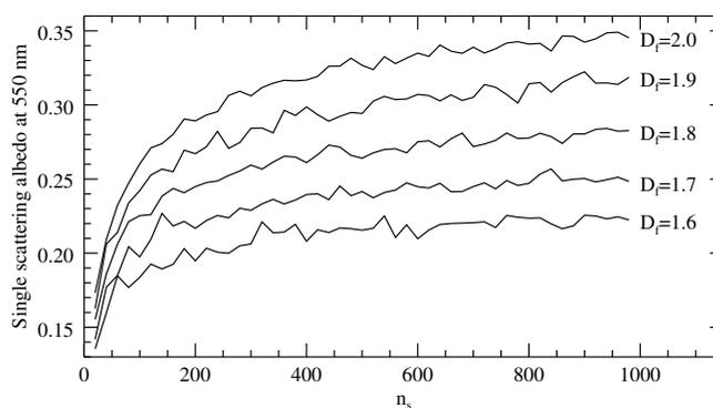
**Figure 3.** The SSA of BCFA at  $\lambda = 550$  nm as a function of  $n_s$  and  $D_f$ . The most likely values of  $D_f$  would be from 1.7 to 1.8, where the SSA values are between 0.2 and 0.3.
