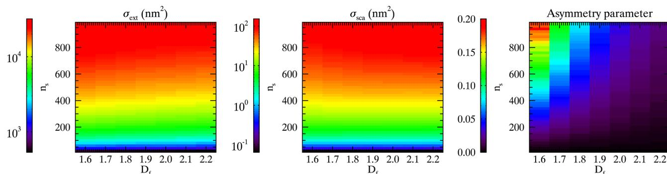
**Figure 6.** Extinction cross section, scattering cross section, and asymmetry parameter calculated using the MSTM code at  $\lambda = 12\mu\text{m}$  for a range of fractal dimensions and numbers of spherules.
