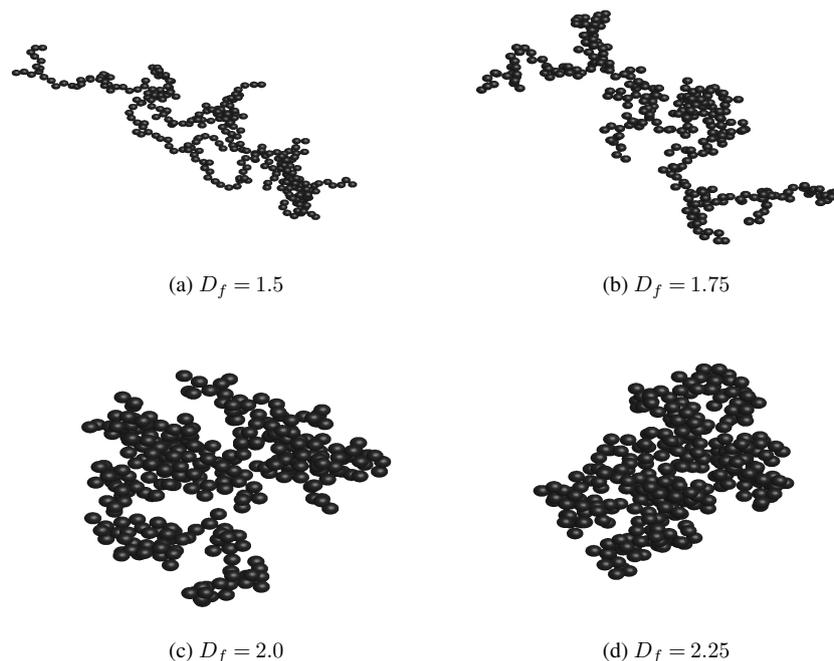
**Figure 1.** Modelled fractal aggregates with  $n_s = 300$ ,  $k_f = 1.25$ , and varying values of  $D_f$ . As the fractal dimension increases, we move from linear to bunched clusters. These aggregates were generated using a cluster–cluster algorithm.
