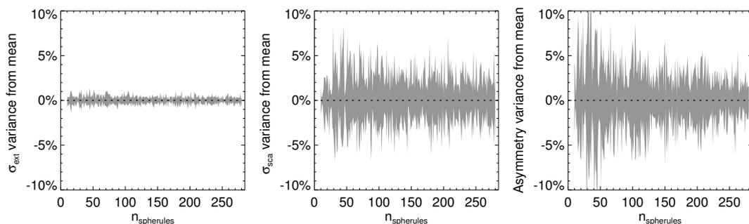
**Figure 5.** Showing the envelope of relative spread from the mean of the three output parameters –  $\sigma_{\text{ext}}$ ,  $\sigma_{\text{sca}}$  and  $g$  – at  $\lambda = 550$  nm for BC with  $D_f = 1.75$ , given four fractal geometries at each size. The high relative differences of  $g$  with low  $n_s$  can be accounted for by the lower values of  $g$  in this regime.
