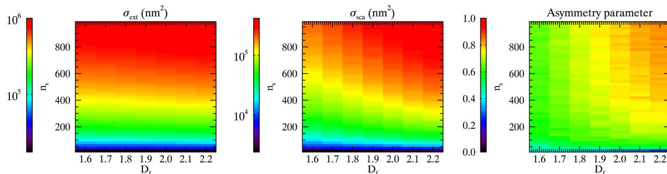
**Figure 2.** Extinction cross section, scattering cross section, and asymmetry parameter calculated using the MSTM code at  $\lambda = 550$  nm for a range of fractal dimensions and numbers of spherules.
