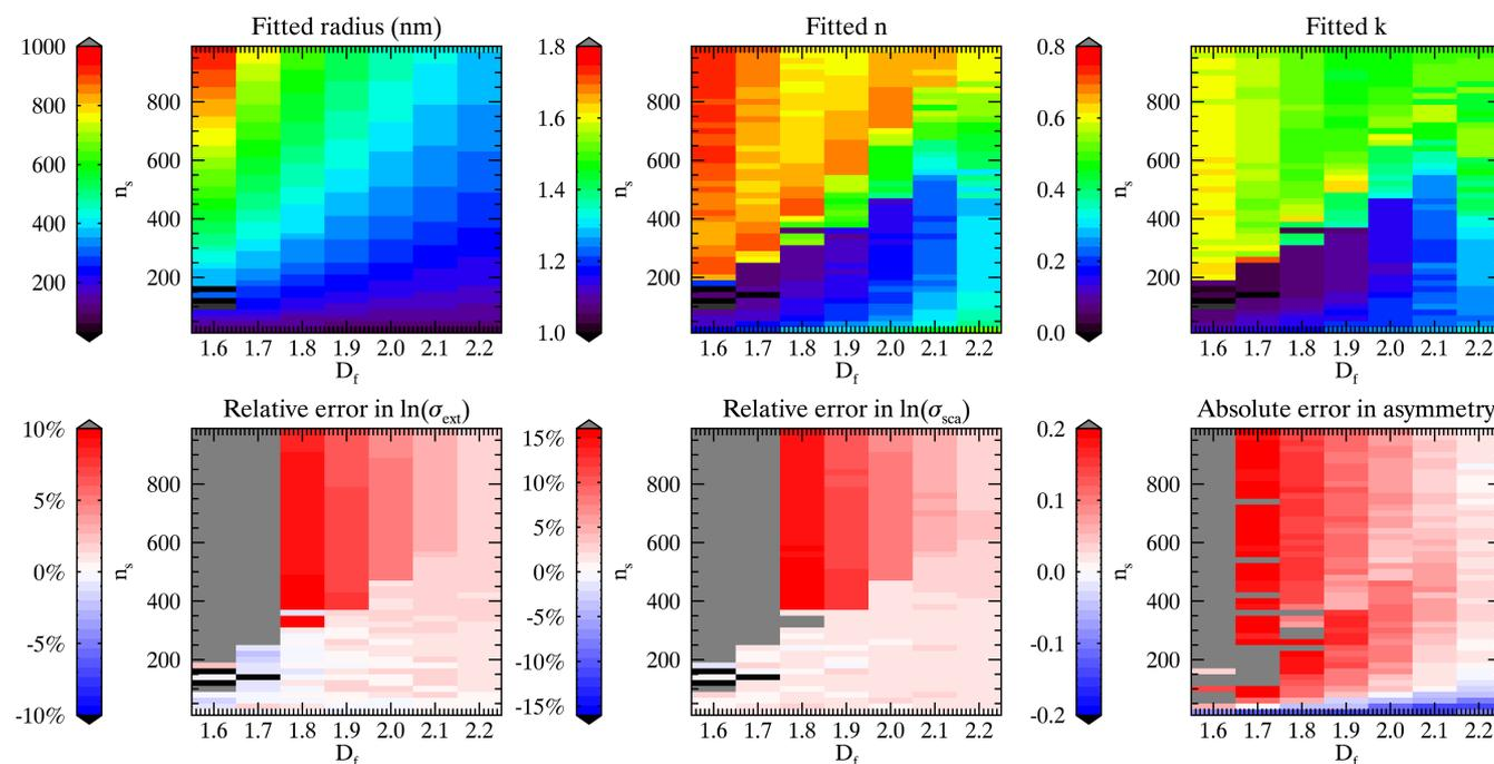
**Figure 8.** The optimum fitted sphere parameters ( $r$ ,  $n$ , and  $k$ ) and their resultant errors relative to the reference MSTM calculations in  $\ln\sigma_{\text{ext}}$  and  $\ln\sigma_{\text{sca}}$ , and absolute errors in  $g$  for BCFA with  $\lambda = 550 \text{ nm}$ . The colour scale has been adjusted so that the very large errors caused by unphysically small BCFA  $D_f$  are clipped.
