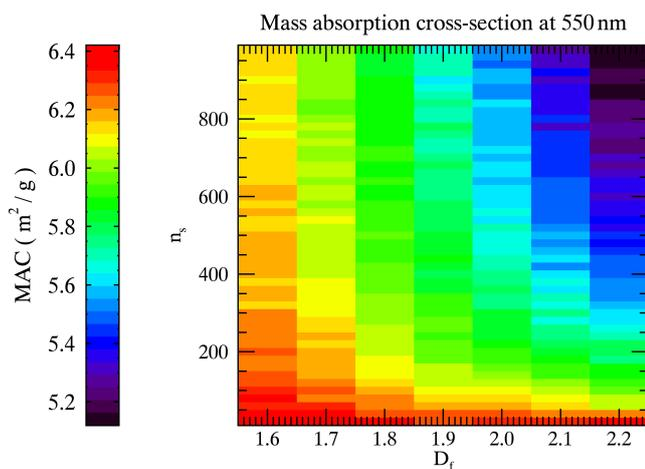
**Figure 4.** The mass absorption cross section at  $\lambda = 550$  nm for BCFAs. This is the absorption cross section divided by the mass of the particles. For these calculations, a density of  $1.8 \text{ g m}^{-2}$  was assumed.
