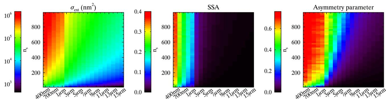
**Figure 7.** Extinction cross section, single scatter albedo, and asymmetry parameter calculated using the MSTM code at  $D_f = 1.8$ . Note the discontinuity in wavelength step size at  $\lambda = 1 \mu\text{m}$ . Unlabelled wavelengths are halfway between the two values on either side.
