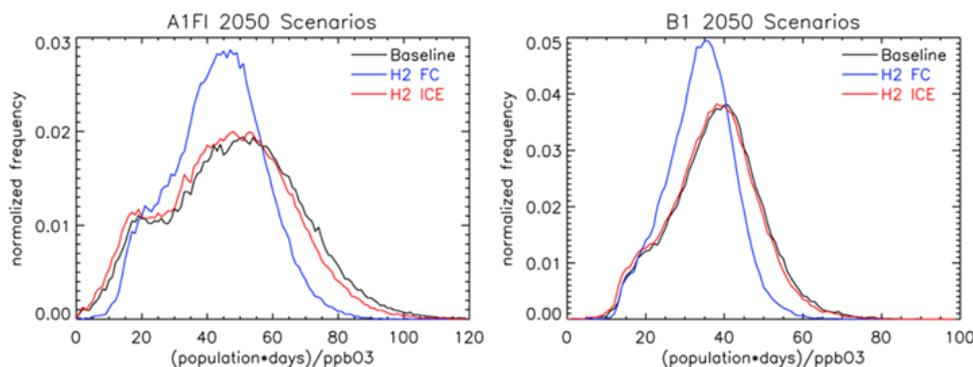
**Fig. 6.** Normalized probability distribution [population-days/ppb] of CMAQ simulated surface daily maximum 8 h-average O<sub>3</sub> concentrations throughout one year for the A1FI (left) and B1 (right) baseline, H<sub>2</sub>-ICE, and H<sub>2</sub>-FC scenarios across the United States. Distributions are based on the US population distribution for 2000 and the bin interval is 1 ppbv.
