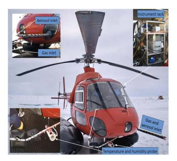
**Fig. 2.** The ASCOS 2008 expedition helicopter with instrument and air inlet locations.
