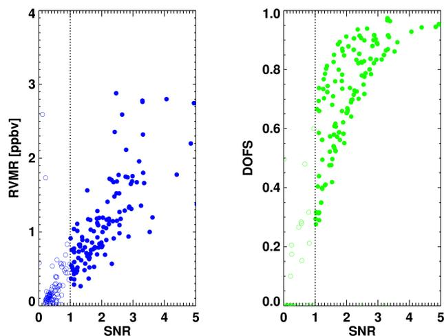
**Fig. 9.** Signal-to-noise ratio (SNR) and degrees of freedom for signal (DOFS) in the TES methanol observations. Left panel: RVMR values as a function of the SNR for a Global Survey from October 2009. Right panel: DOFS as a function of SNR for the same Global Survey. Empty circles have SNR < 1.0.
