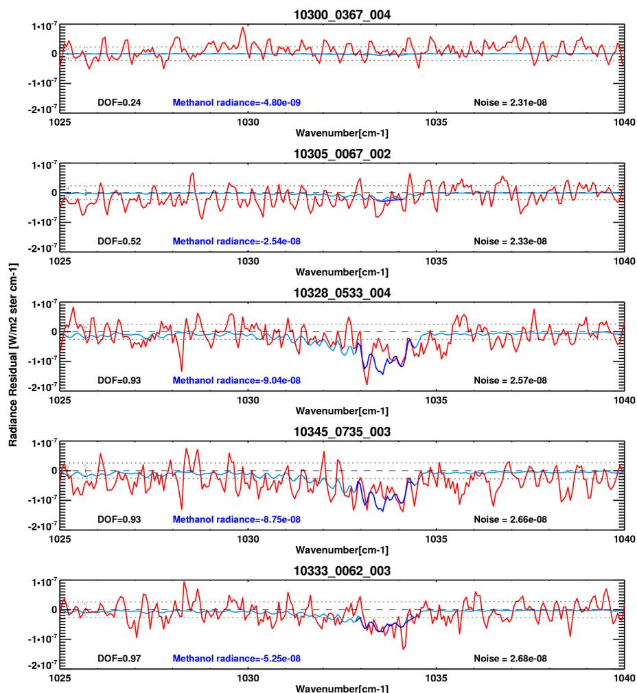
**Fig. 8.** Methanol spectral signal in the TES observations. Shown are sample differences between measured TES spectra and forward model runs with no methanol (red curves), and the corresponding differences between forward model runs with retrieved methanol and no methanol (light blue curves). The methanol radiance is the mean of the latter over the spectral range highlighted in dark blue. The dotted lines indicate the expected noise level.
