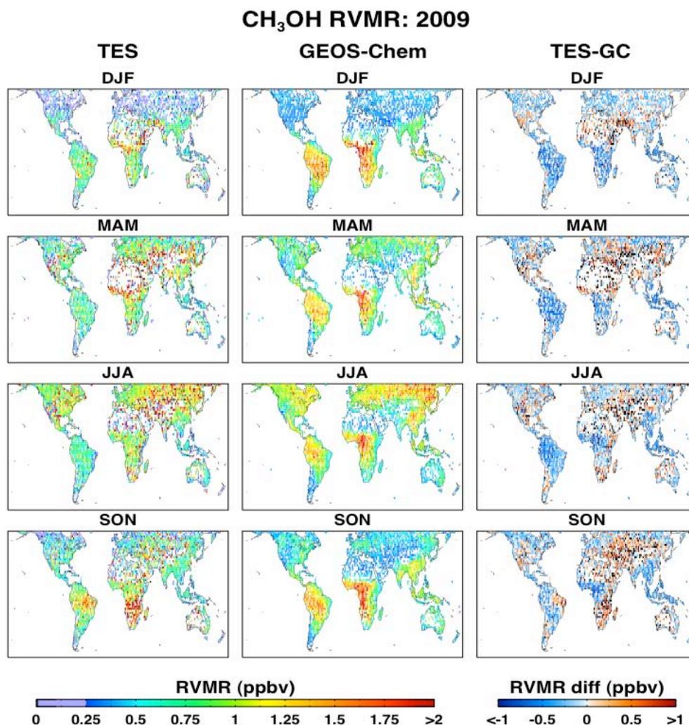
**Fig. 11.** Seasonally averaged CH<sub>3</sub>OH RVMR on a 2×2.5° grid for 2009. Left panels: retrieved values from TES. Middle panels: simulated values from GEOS-Chem with TES averaging kernel applied. Right panels: TES-GEOS-Chem.
