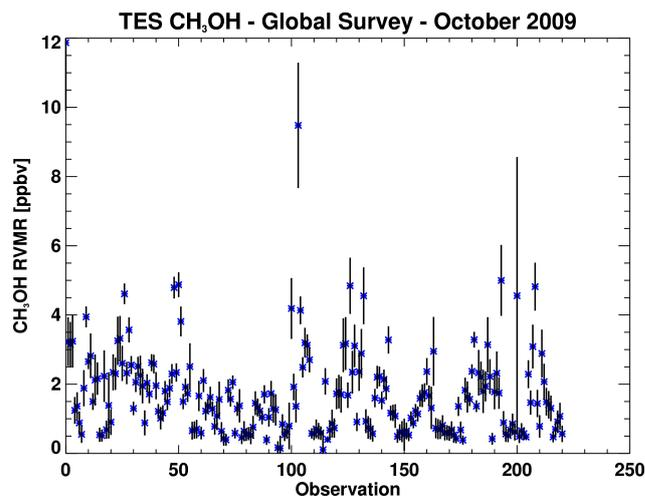
**Fig. 10.** Sequence of retrieved methanol RVMR values from TES for the October 2009 GS used in Fig. 9. The x-axis values are simply an index indicating order in time. The error bars include both noise and smoothing error.
