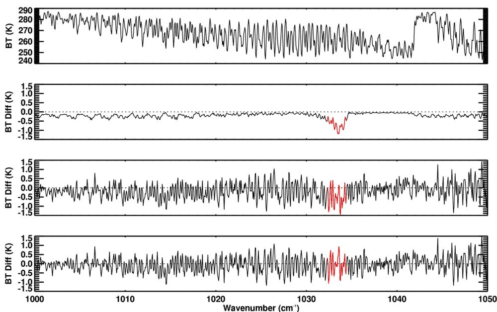
**Fig. 5.** Sample TES methanol measurement over central Canada (59.34° N, 106.52° W) on 23 June 2008, which coincided with the second phase of the NASA ARCTAS campaign. Top panel: spectral brightness temperature observed by TES. Second panel: CH<sub>3</sub>OH signal, obtained by differencing third and fourth panels. Third panel: measurement-model residuals based on the initial guess methanol profile. Fourth panel: measurement-model residuals following the methanol retrieval.
