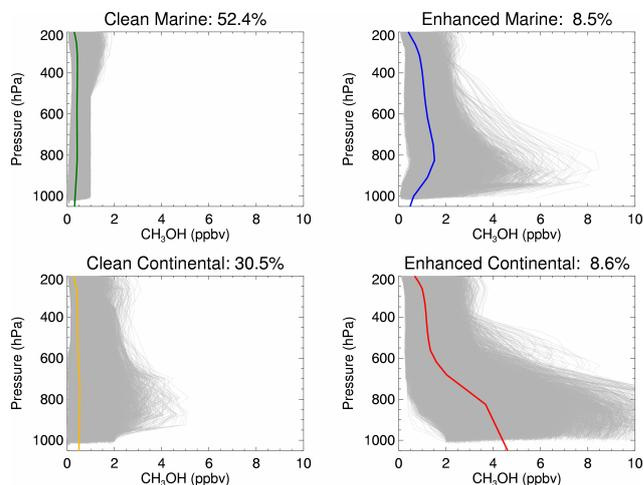
**Fig. 3.** Methanol profiles simulated by GEOS-Chem over the entire globe for 2004 binned by type (in grey). The mean profiles for each category, shown in color, are used as a priori profiles in the TES methanol retrieval. See text for details.
