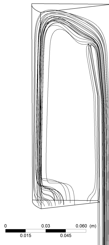
Fig. 1. A 30^\circ radial section is used to model the flow through the inlet assembly with CFD. Air at -40^\circ\text{C} and 1\text{ }\mu\text{m} diameter particles (density of 1000\text{ kg m}^{-3} ) are introduced through the opening at the bottom of the inlet. The outer surface and the inlet pipe in the centre (ending in a funnel at the top) are heated to 20^\circ\text{C} . Trajectories of the 1\text{ }\mu\text{m} particles are depicted as grey lines.
